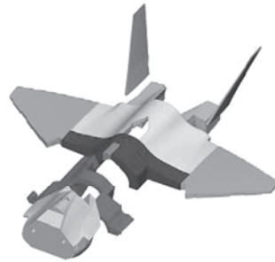
Figure 3.10 Joint strike fighter fuel tank layout (Courtesy of BAE Systems) (See Colour Plate 2)
