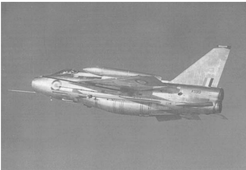
Figure 3.18 Lightning F6 with over-wing tanks (Courtesy of BAE Systems)
